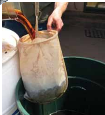
Before using cooking oil in a car as a fuel, chunks of food present in the oil need to be filtered out.
